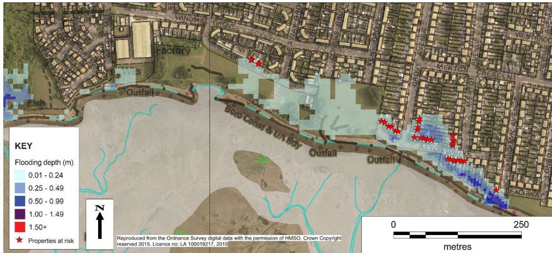
Figure 3: Modelled flood extent, depth and properties at risk during a 1 in 100 year event in 2015
